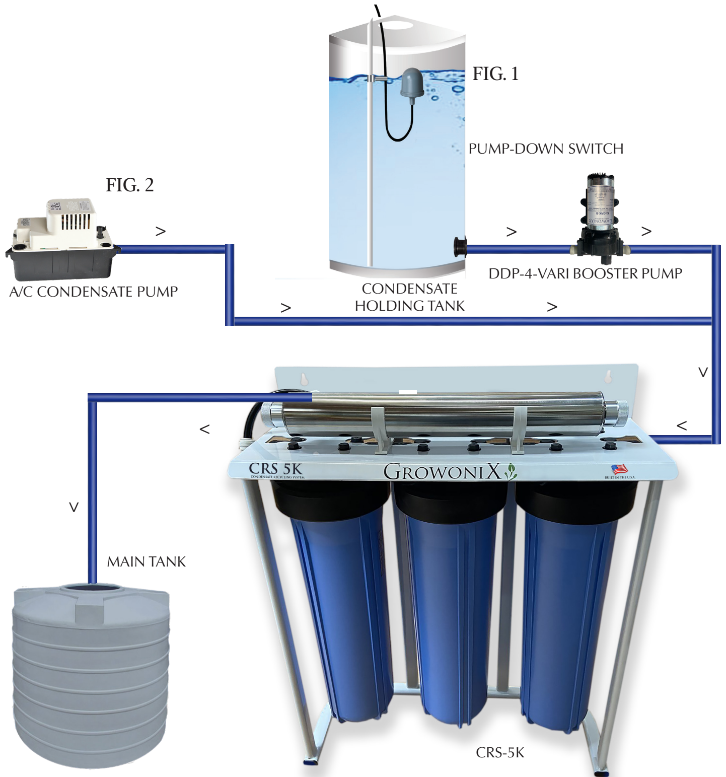
Fig. 2 Diagram of A/C condensate pump to CRS-5K setup
