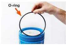
Clean o'ring and o'ring seat, then re-grease with food grade silicon grease.
