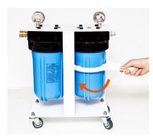
Unscrew sediment and carbon filter housings using supplied filter wrench. Wash inside of filter housings to remove debris.
