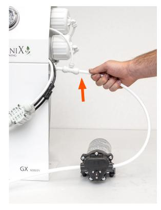
Insert the 3/8" pump output tubing into the RO filter input.
