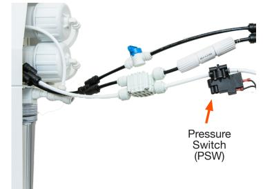
Install the pressure switch on the product water line (RO out tubing) after the auto-shutoff valve. The switch can be installed in any direction.
